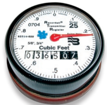
Each dial rotation equals one cubic foot or 7.48 gallons.
